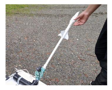
6. Pump the bike pump until the pressure reaches 30psi.
